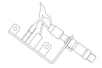
FIGURE 10. Incorrect Shape of Pilot Flame
